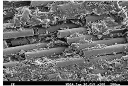
Fig. 6(b): Worn Surface of 5 % NanoSic
