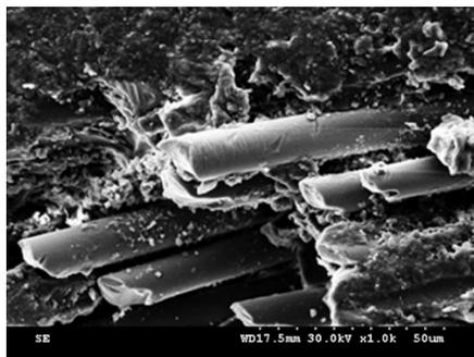
Fig. 6 (a): Worn Surface of 1% NanoSic
